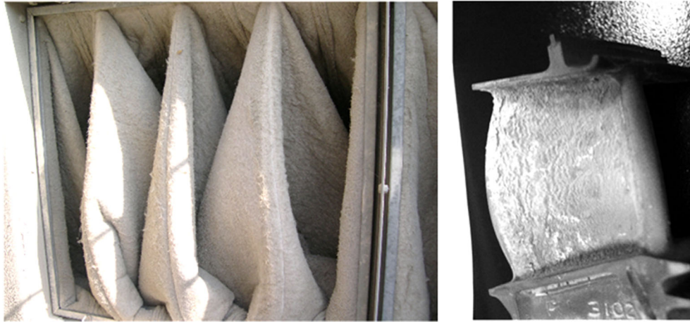
Turbine blade with thick deposits of limestone dust
