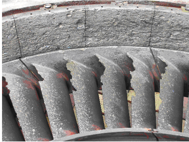
Figure F.3—Gas Turbine Damage from FOD
